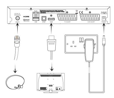
Connect the cable from your dish to the LNB IN socket at the back of the receiver (if the dish cable is fitted with a wall socket inside your home, you will need a connecting cable, which you can get from your installer).
