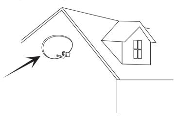
To receive freesat, you must connect your Plaza HD•S receiver to an appropriate satellite dish, fixed in position and accurately pointed at the 28.2° East satellite position.
